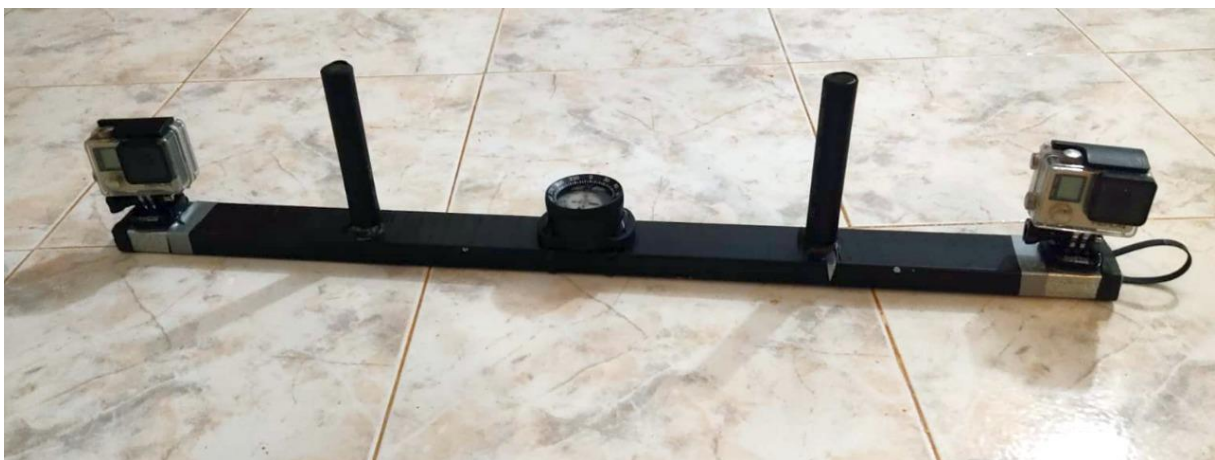
Figure 2. Camera mount for stereo-video transects. Technical details: base separation- 70mm, inward facing angle of 8°. Fitted with compass to navigate underwater and adjust and control swimming direction during transects.
