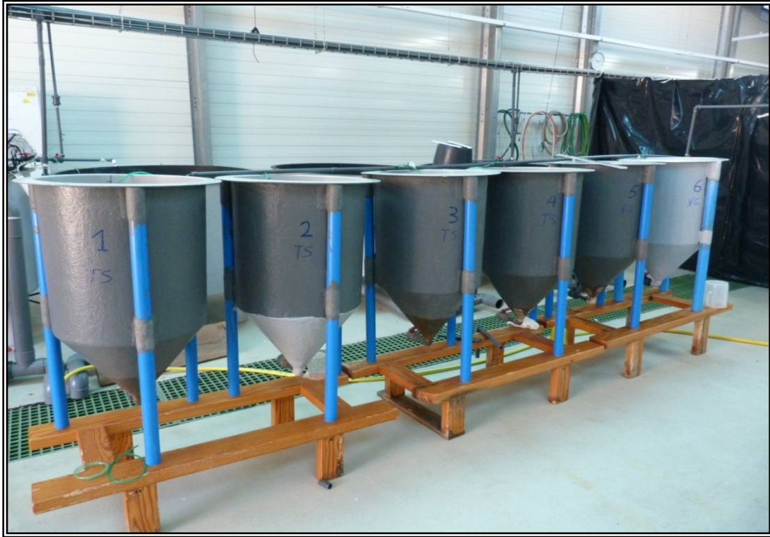
Figure 5. 100 L cylinder-conical fiberglass tanks used for Artemia spp. culture.
