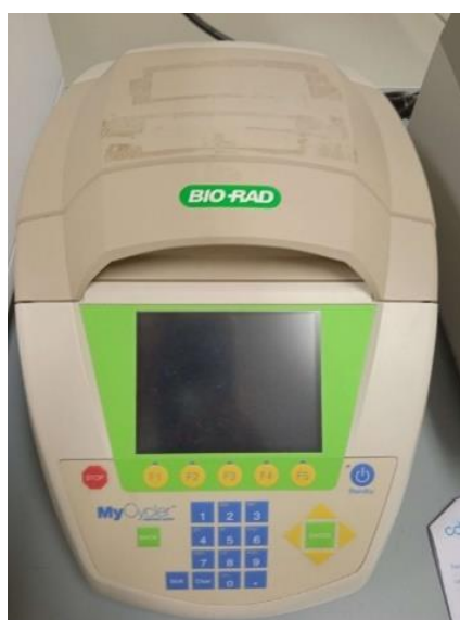
Figure 3.5-Thermocycler MyCycler (Bio-Rad Laboratories, USA) used for polymerase chain reaction.
