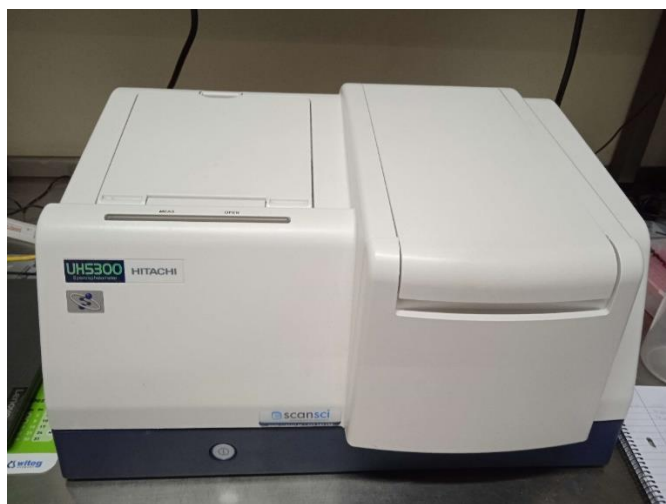
Figure 4.10- Double Beam Spectrophotometer UH5300 (Hitachi, Japan) used for determination of nitrate concentration.
