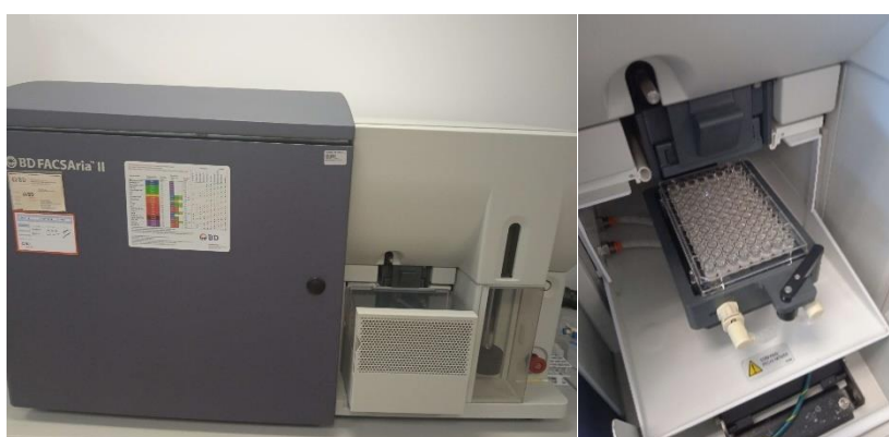
Figure 3.2-Flow cytometer BD FACSAria II (Becton Dickinson, USA) (Left) used to gather samples in a 96-well plate (right).
