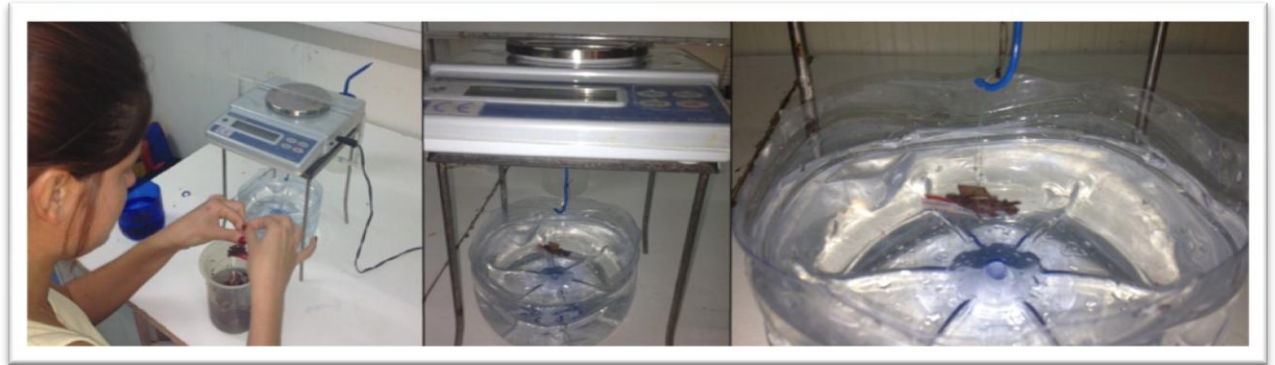
Figure 3.3. Buoyant Weight Technique in the field station Ramalhete, where tagged rodolith were measured in the seawater using the balance.
