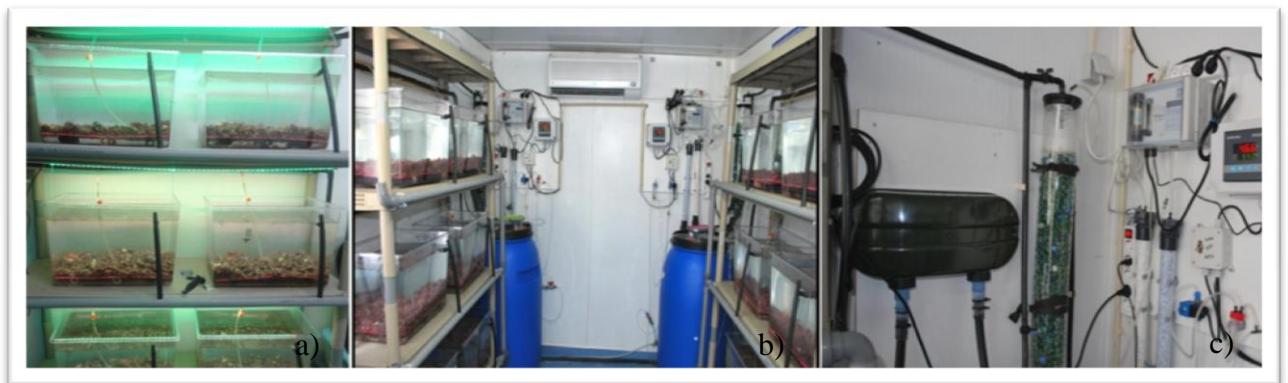
Figure 3.2. Aquariums and mesocosm in the Ramalhete field station; a) six aquariums in each system with controlled level of CO 2 , b) two mesocosm systems with blue tanks where seawater
