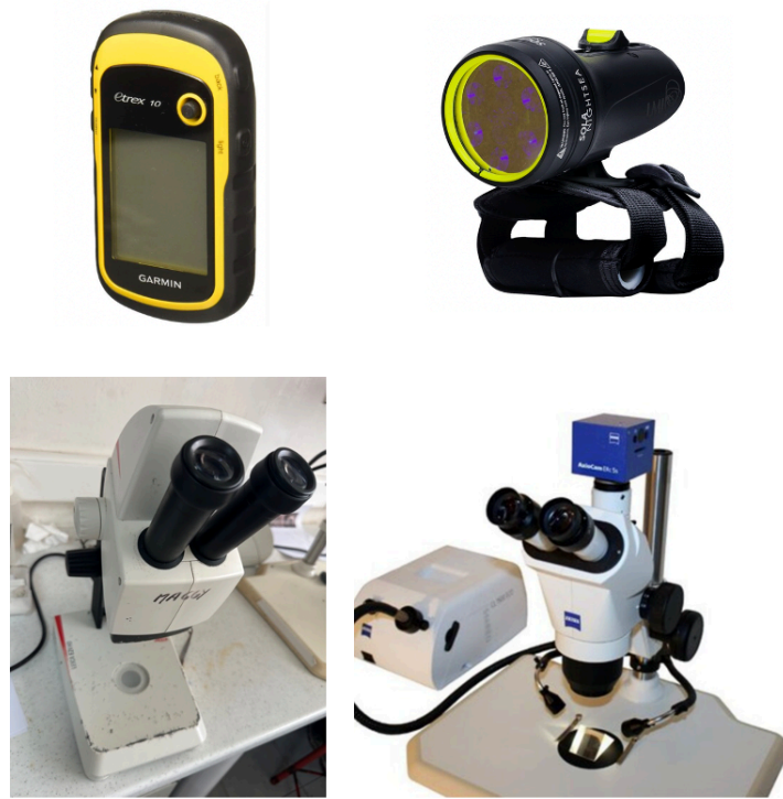
Figure S1: Equipment used for research, analysis and photography of study organisms (Coral reefs, CCA, Macroalgae). (A) Garmin Etrex 10 GPS. (B) Sola NightSea UV light. (C) LEICA EZ4 HD Binocular Lens. (D) Zeiss Stemi 2000-C 6,5 50x.6,5 50x ZOOM.
