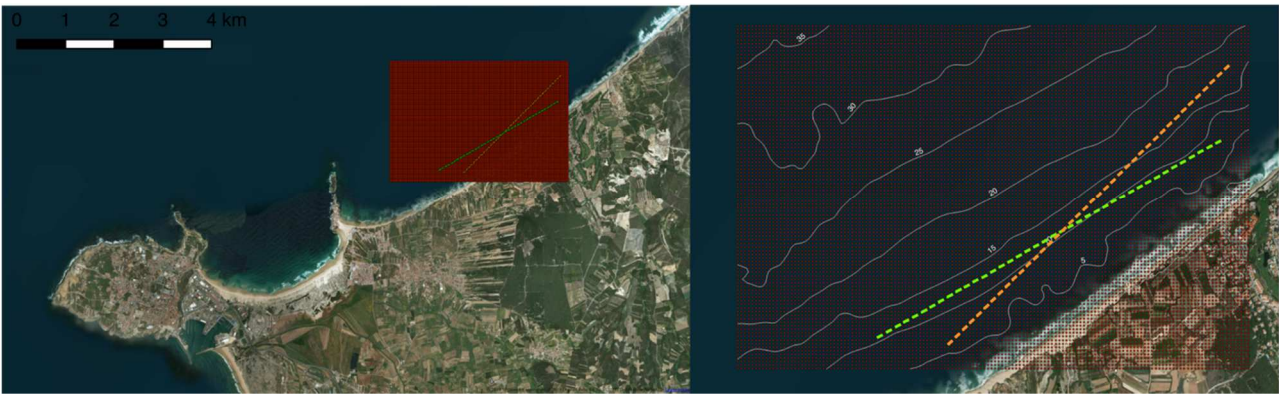
Figure 4.24 Location and disposition of the wave farm of 40 WECs of WaveRoller kind. The orange WECs refers to the configuration perpendicular to the incoming waves of 315° while the green WECs refers to the same configuration rotated of 30°.
