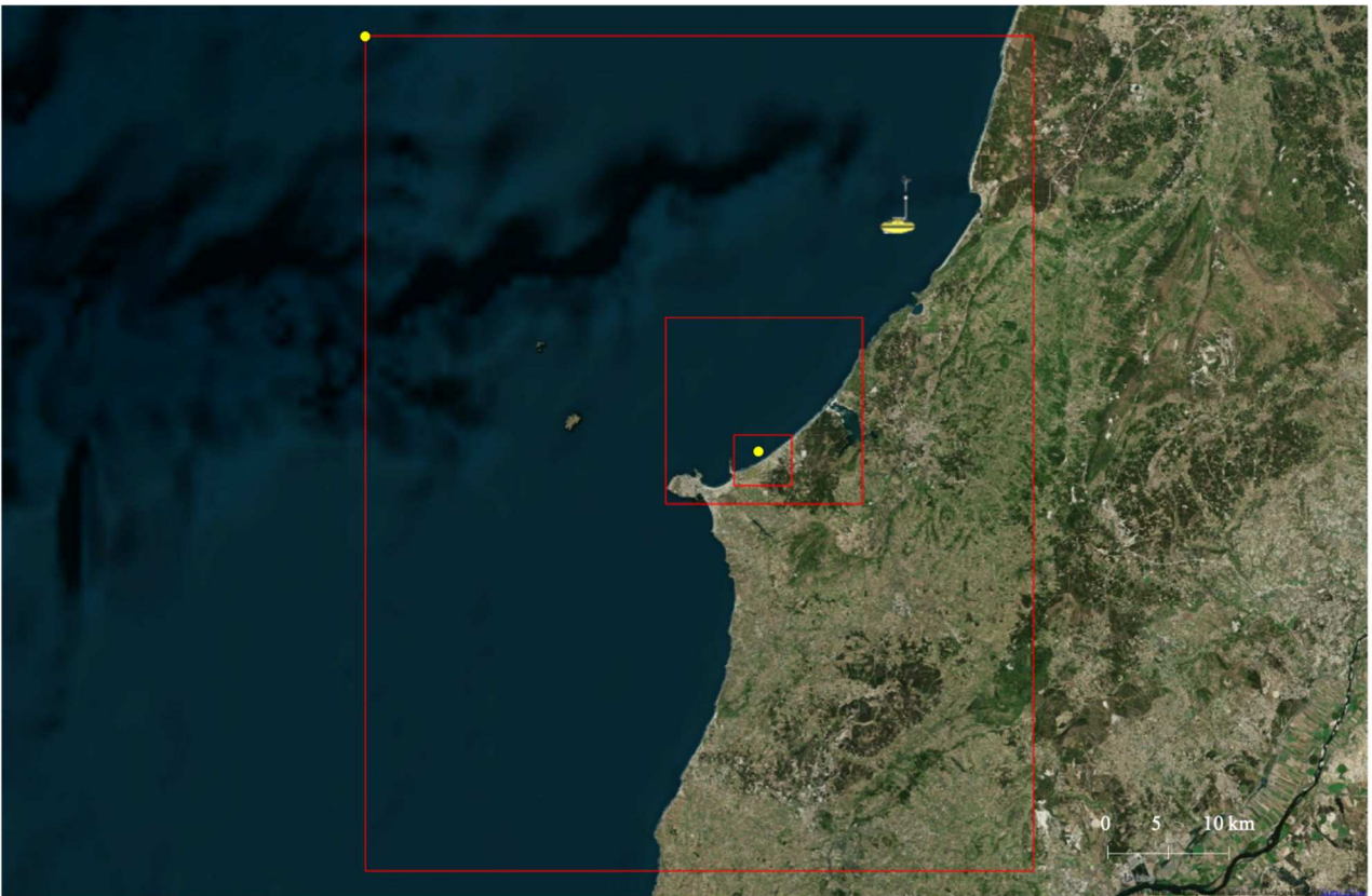
Figure 3.3 Computational grids for SNL-SWAN simulations: the most external one is the main grid and the two insides are the nested grids. The points where the wave climate has been characterized are reported (yellow circles) along with Nazaré Costeira buoy.
