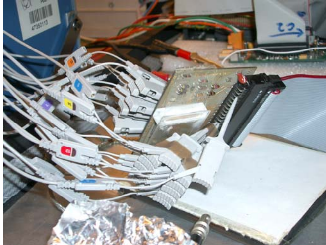
Figure 4-11: Photograph of the Omega3/LHC1 chip test card (see figure 4.5) connected with the logic analyzer probes.
