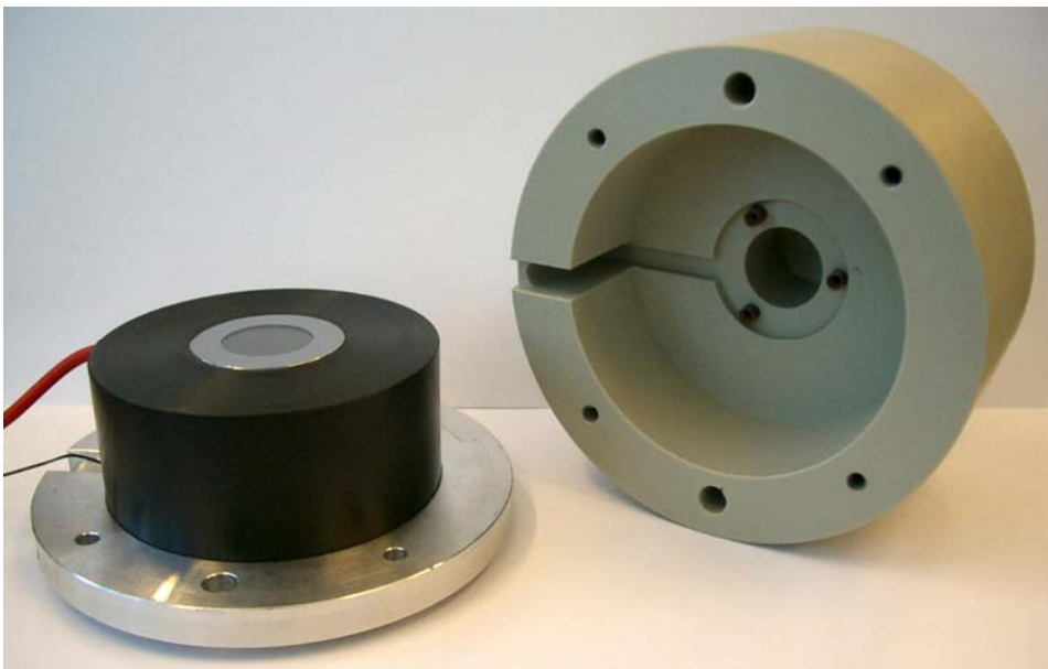
Figure 3-23: Photograph of the proximity focusing tube and the polypropylene casing. This HV shield casing has a centered hole to adapt the collimator. Three springs are visible around it and they are useful to lean the collimator on the scintillator. The groove cavity is for the tube and collimator high voltage cables.
