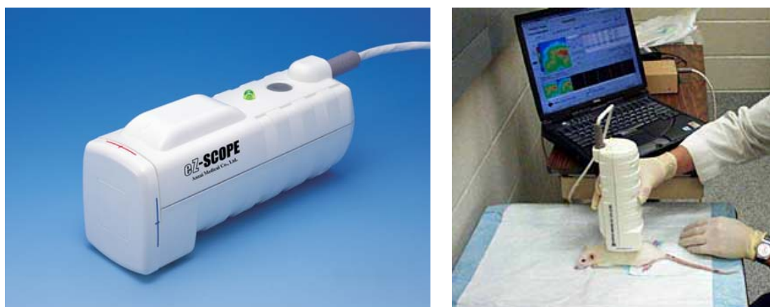
Figure 2-6: (left) Photograph of the eZ-SCOPE AN portable gamma camera; (right) Imaging application of gene expression in a representative mouse.
