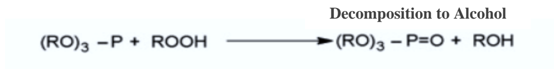
Figure 1.16 Decomposition of hydroperoxides by organophosphorus. Adapted from: (Shanina et al., 2002)
