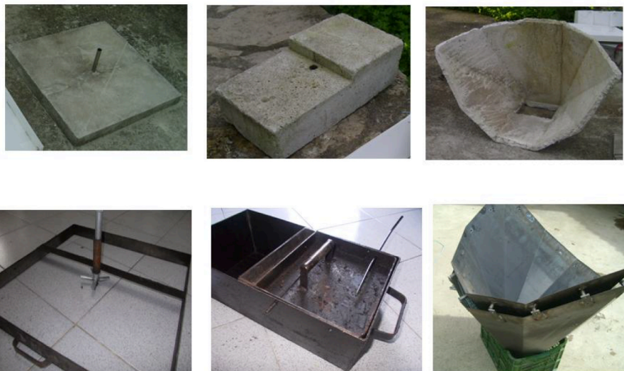
Fig. A1. Moulds and concrete pieces of the Pucca solar cooker.
