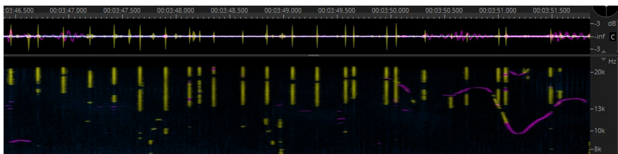
Figure 1.1 - Spectrogram of recording with T. truncatus vocalizations. Pulsed signals (clicks) can be seen in yellow. Narrow-band tonal sounds (whistles) can be seen in pink with a range from around 9 kHz to around 16 kHz; the lower end of a harmonic can also be seen around 20 kHz; the rest of the harmonic would be outside of the recording range.
