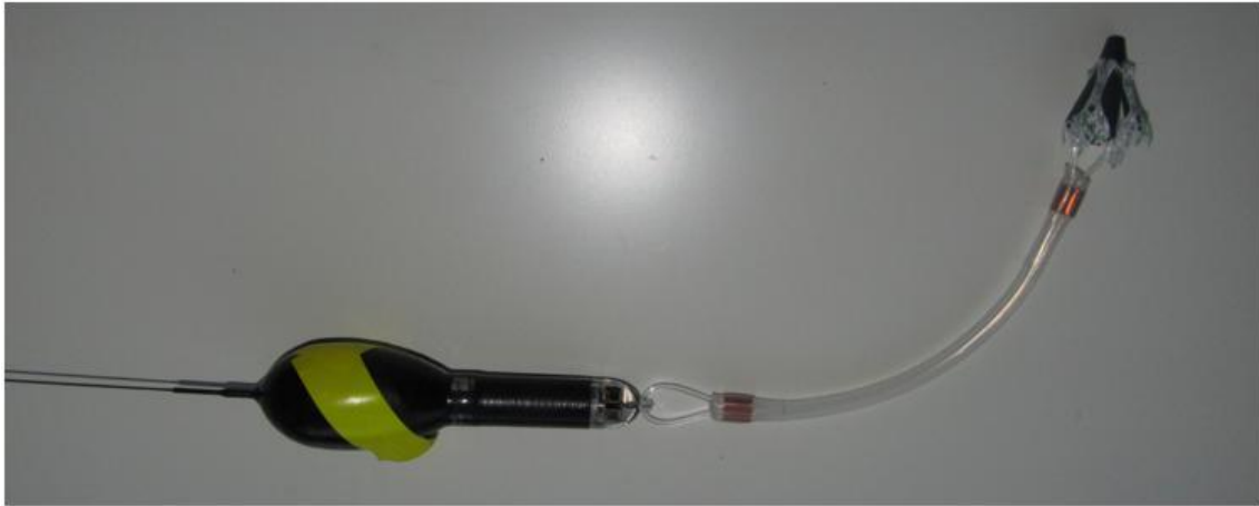
Figure VI.1: Pop-up Satellite Archival Tags (PSAT) used in this study. Type PTT-100 X-Tag built by Microwave Telemetry Inc.
