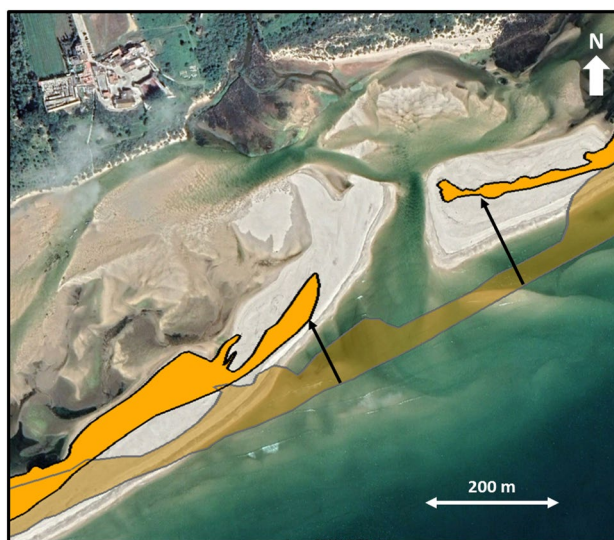
Figure 4. Oceanic coastline retreat and inland inlet migration between 2007 (before inlet opening; transparent orange) and 2021 (opaque orange). The orange areas in the image represent the vegetated (dune) area at the barriers. The arrows show the higher retreat near the inlet. Image source: Google Earth, May 2021.
