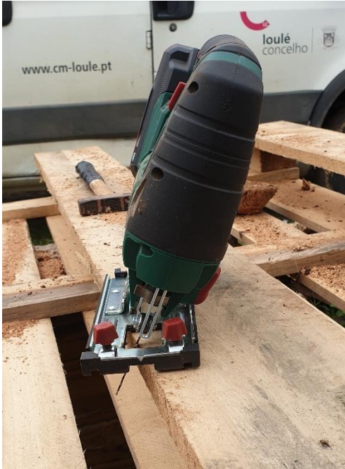
Figure 18. Jigsaw calibrated with angle (Picture taken by author on 24.11.2022)
