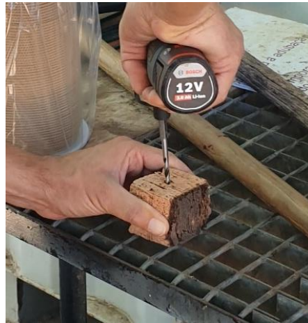
Figure 21. Perforating distance cubes with wood drill (Picture taken by author on 26.07.2022)
