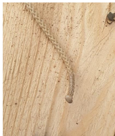
Figure 20. Rope end after being sealed with blowtorch (Picture taken by author on 24.11.2022)
