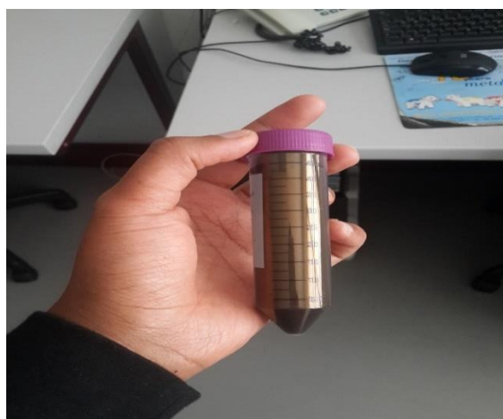
Figure 11 Gold film and precipitate on the side wall and bottom of falcon.
