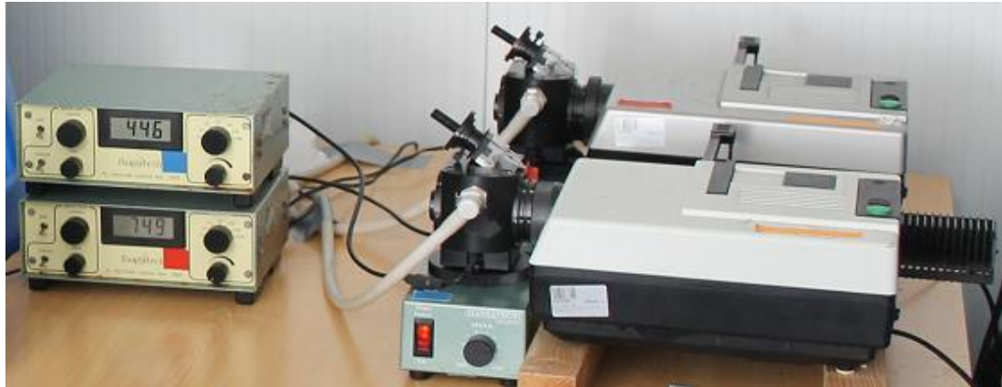
Figure 7: Clark type oxygen electrode. Connection of incubation chambers to light sources.
