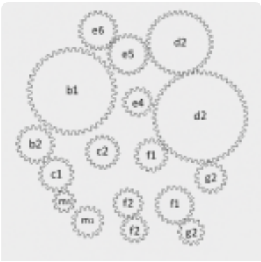
Fig 3: Schematic reconstruction of the gears based on CT projections.
