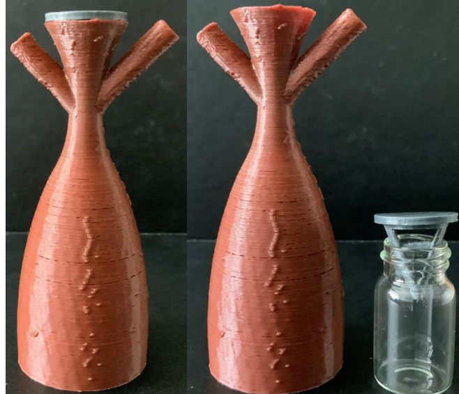
Figure 5.11 – The first 3D printed device. On the left, the device if fully assembled, and on the right, the two parts are separated, with the weighing chamber on the side.
