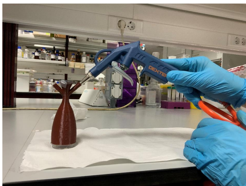
Figure 6.3 – Air compressor used to pump air into the device, with the aim of dragging the powder to the petri dish in the bottom.
