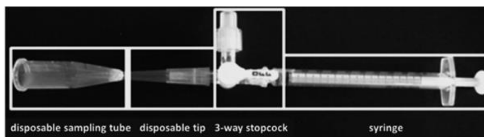
Figure 1.10 – Apparatus for dry powder dispersion. From left to right: an Eppendorf tube functioning as a disposable sampling tube, connected to a 3-way stopcock by a disposable tip, and on the right end, a 1 mL syringe. From [218].
