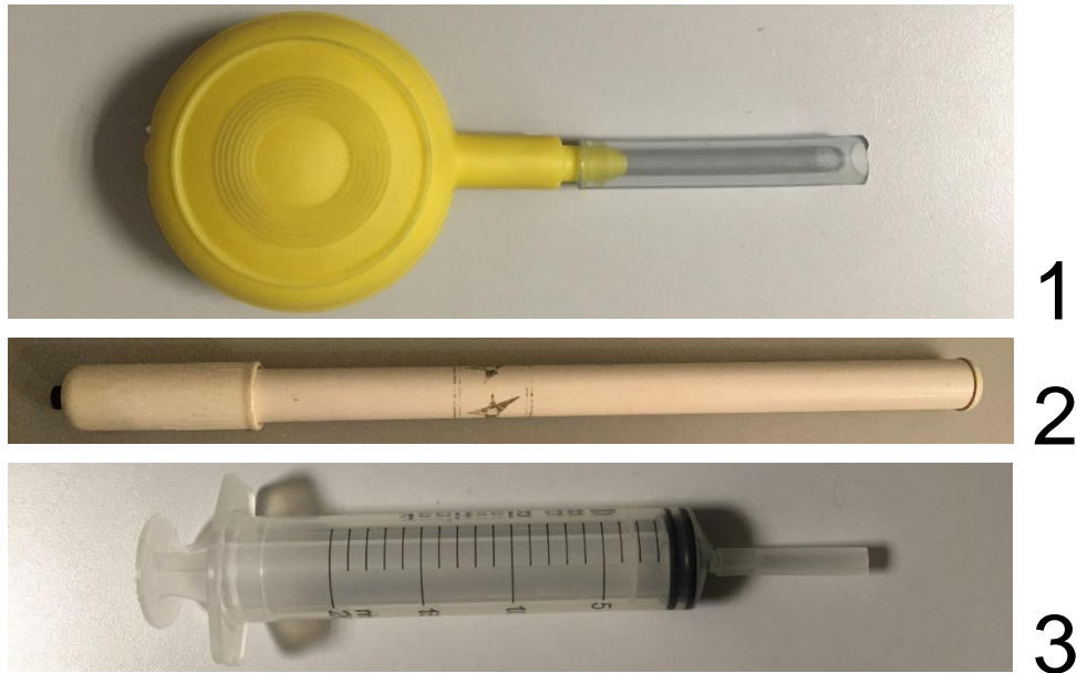
Figure 6.1 – First three pumps tested for the insufflation of powders with the device. From top to bottom: the lens blower (1), the bicycle pump (2) and a syringe (3).
