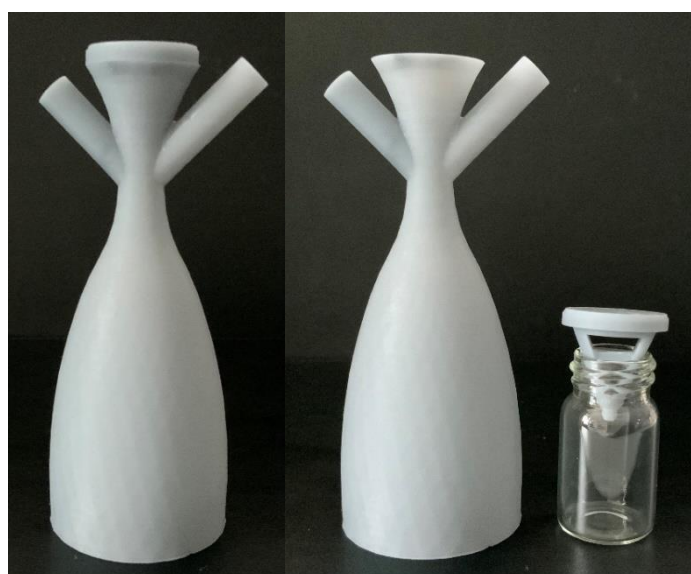
Figure 5.13 – New device printed by stereolithography using UV light and a washable resin.
