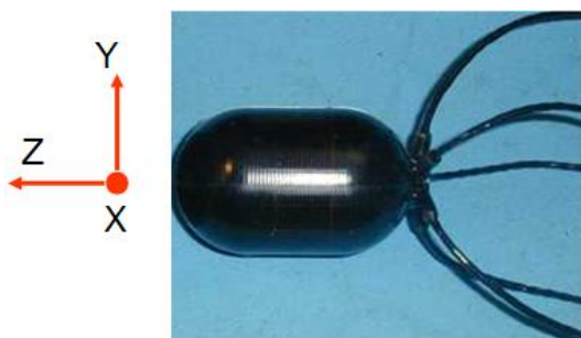
Figure 4.5: Constitution of a single vector sensor and x , y and z -axis orientation.
