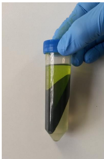
Figure 3.4 - Three phases were obtained, through liquid-liquid separation (hexane and water) of the crude lipid extract. Near the top of the Falcon tube, one can see the hexane fraction. The colloidal fraction and the water fraction can be observed in the middle and at the bottom, respectively.
