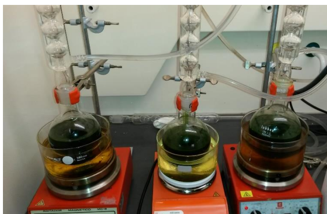
Figure 3.3 - Lipid extraction experimental setup. Wet microalgal biomass and ethanol were added to round bottom flasks, partially submerged in a paraffin bath, maintained at reflux temperature (~70 °C) and stirred for three different periods with the following durations: 2 h, 30 min and 15 min.
