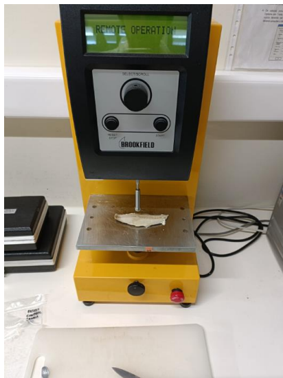
Figure 2.7 - LFRA Texture Analyzer used in hardness tests.
