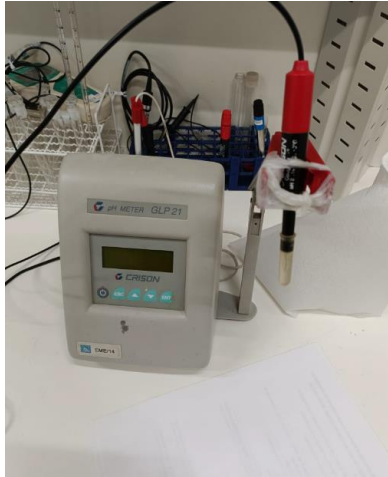
Figure 2.8 - pH meter and semi-solids probe used for pH readings.
