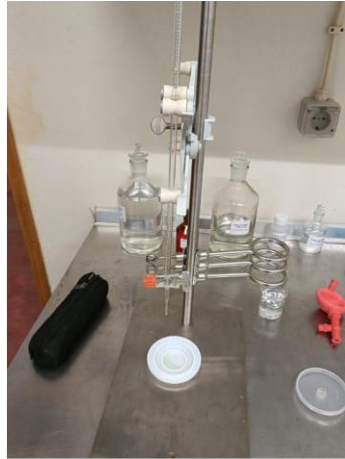
Figure 2.12 - Titration process used to determine TVBN.
