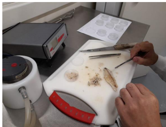
Figure 2.9 - Hygrolab (Rotronic Instruments, UK) probe and readings display (left), reading cells and fillet mincing (centre and right).
