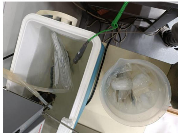
Figure 2.4 – Top view of thermostatic water bath (left) used for cooking the mackerel fillets, and water and ice bath used to cool down samples (right).
