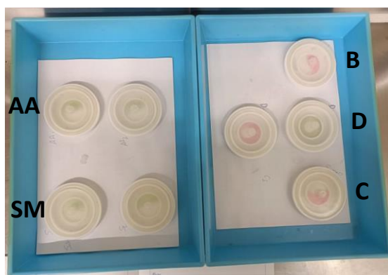
Figure 2.11 - Conway cell after heat treatment (B is blank, D is control of diffusion, C, AA, and SM are the samples).
