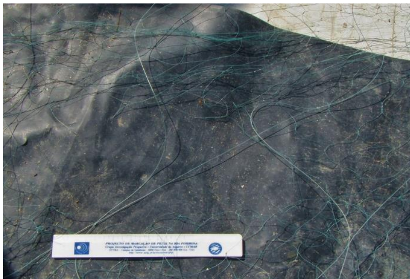
Figure 2.3.1. Net damage assessment with the 20 cm ruler on a hole on the upper layer and inner mesh.
