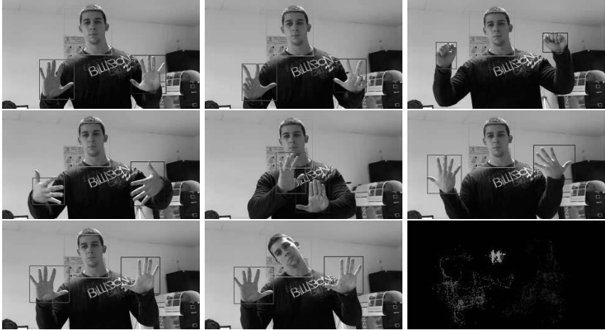
Fig. 2. The optical flow model applied to a person while performing several hand and head gestures. Hands and head are marked by their bounding boxes. The bottom-right image shows the combined centers of the boxes.
