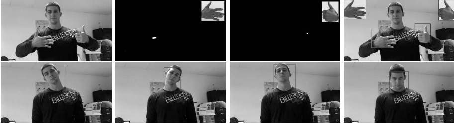
Fig. 4. The top row illustrates hand gesture recognition: input image, thresholded probability maps of the two detected gestures with their peaks in white, and the final result. The bottom row shows examples of the recognition of four head poses: right, left, up and down. Along the vertical edges of the bounding box, the two green points show the average location of skin-colored pixels.
