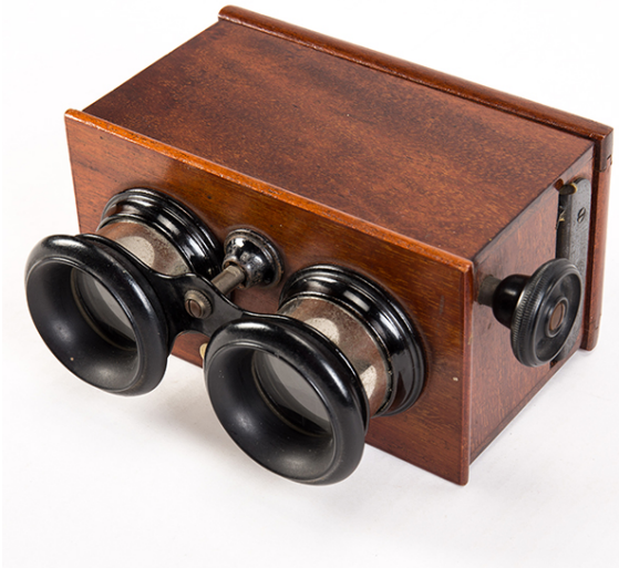
Figure 2. Portable stereoscopic viewer from the late 19th to early 20th century. © Wikimedia commons
