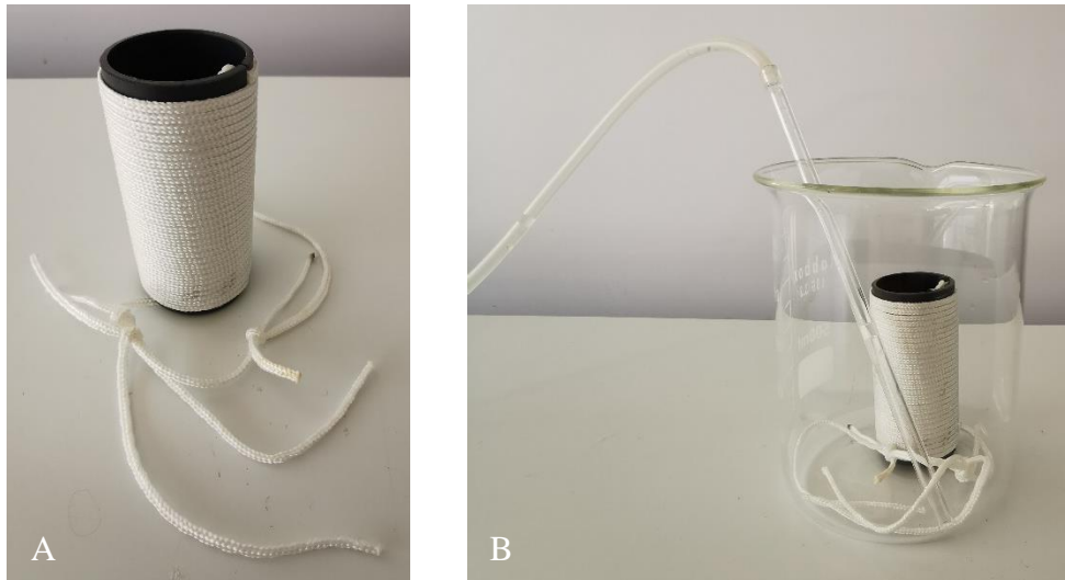
Figure 2.1 A) spool photo; B) aerating system photo.
